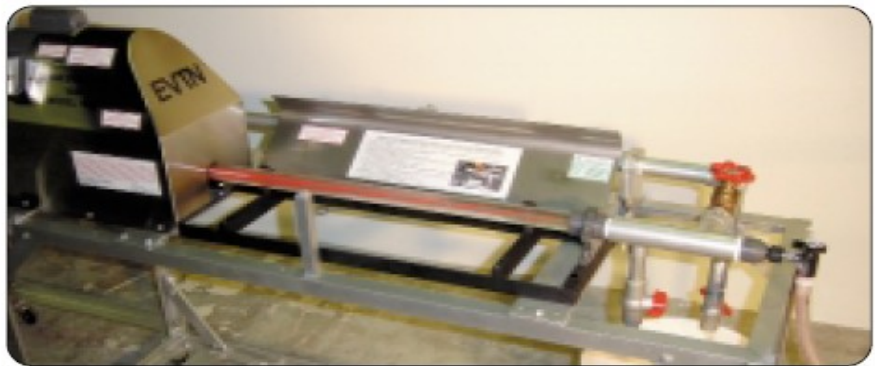
An 8 gallons per minute throughput Voraxial Separator in use at a North American oil refinery, showing very clearly the separation between oil and water in the vortex. Other models of the Separator can handle throughputs in excess of 5,000 gpm.
