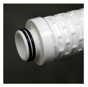
The standard Oilblock cartridges will absorb 2ltr of oil before it reach its change out differential pressure of 2.5 bar. This unique cartridge blocks after saturating which is a very simple and effective indication for change out prevent any bypass of oil.
